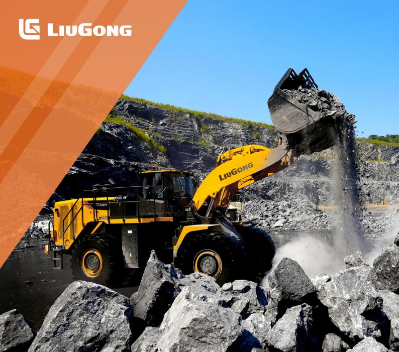
**Cummins X15 Engine** 432 kW (580 hp / 587ps) @ 1,800 rpm **Max Gross Power** 411 kW (552 hp / 559 ps) @ 1,800 rpm **Max Net Power Operating Weight** 52,000 kg **Standard Bucket Size Standard Breakout Force** 3,915 mm **Standard Dump Clearance**
